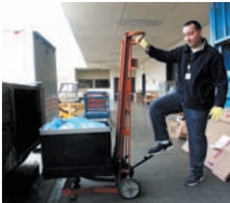
A hydraulic pump operated by a foot pedal raises the compacted garbage to waist height.
