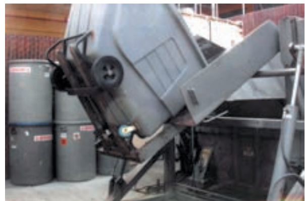
Stationary tilt truck/hopper dumper. Trash is dumped at the push of a button.
