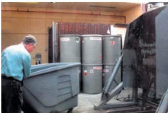
Stationary tilt truck/hopper dumper. Trash is dumped at the push of a button.
